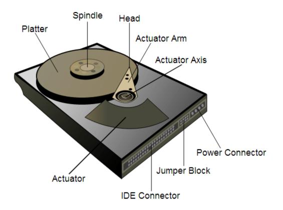
Actually, the files on the hard drive are all scattered on the platter in **sectors** and **tracks**. (Tracks are concentric circles, and the pie-shaped wedges present on each track are called sectors.) Also, the data flow control from and into the Hard Drive is controlled by the operating system.
